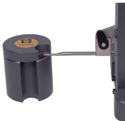
Taking the probe constant value with the setting gage 54-930-202
