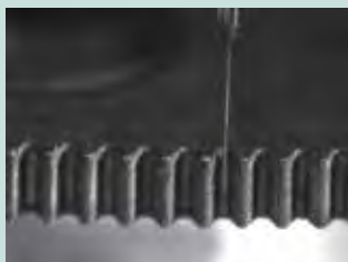
Measuring form of micro gear teeth
