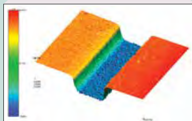
3-dimensional topographical result, data of micro-circuit
