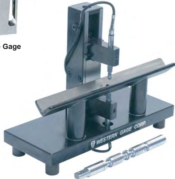
Vee Gage checks hydraulic valve spool O.D.s utilizing opposed set of LVDT Probes.
