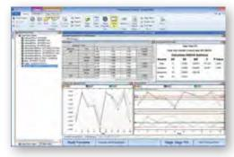
In addition to the standard calculations, the software provides graphical tools for analysis of the measurement system. The Xbar and R chart can show whether there is adequate gage discrimination to record part to part variation in production and if operators are consistent. The Part-by-Appraiser plot can show if there is a lack of consistency between operator inspection techniques.
