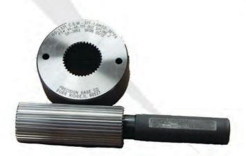
We also manufacture Taper Master Plugs (TMPs). A TMP is used for the manufacture and checking wear condition of ring gages. A TMP has three lines inscribed as depicted in the diagram below; a new ring will be manufactured to fit between the first two lines. When the ring passes over the third line, the ring is worn.
